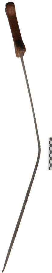
Figure 4. A replica sword bent in the middle part (photograph by the author).
