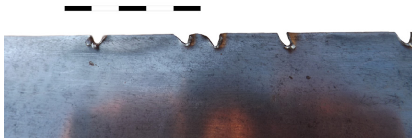
Figure 5. Notches with warping on the medio-distal region of a Celtic sword replica (photograph by the author).
