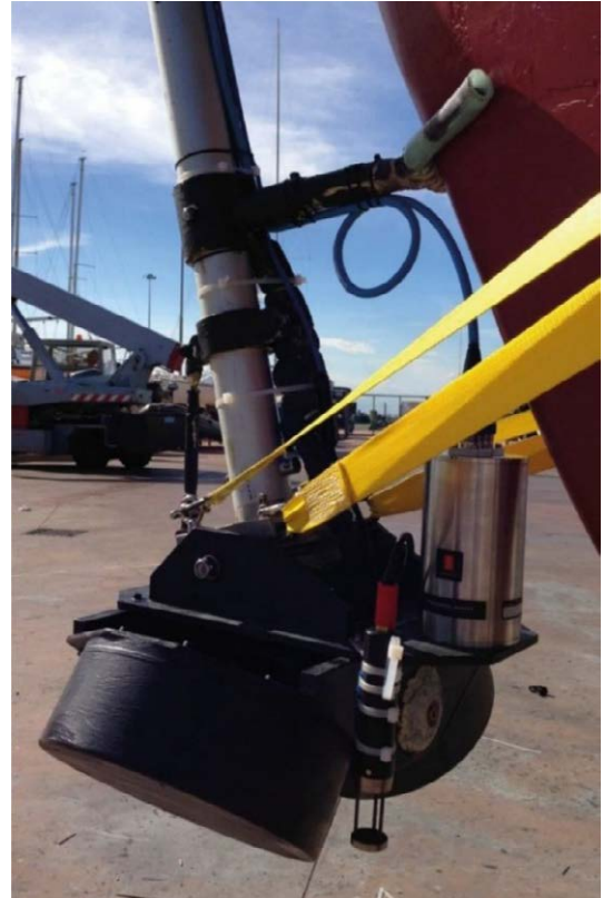
Figure 2. The CNR-ISMAR vessel Litus, above, mounting the multibeam echosounder system Kongsberg EM2040DC used for the morphobathymetric survey, on the right.
